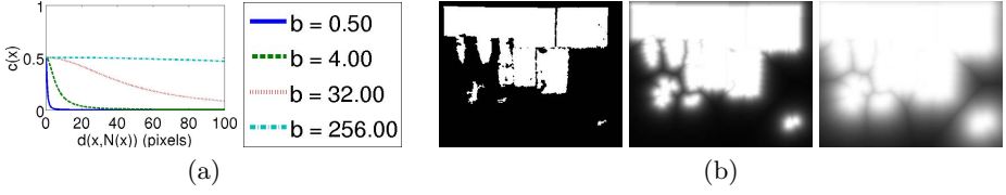
Fig. 2. The role of confidence values. (a) c(x) vs d(x, N(x)) for \psi = 1 and varying b ; (b) c(x) plotted for Fig. 1(bottom) with \psi = 0 and b = 1, 10, 32 (l. to r.).
