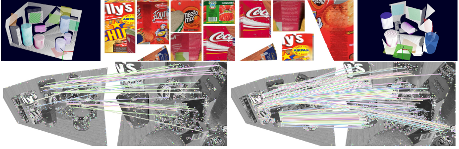
Fig. 4. Wide baseline matching for a synthetic setup. (top row) Outer left and right image illustrate the found models in the 2.5D point cloud; images in-between show developed textures. (bottom row) SIFT matches consistent wrt. the underlying 6DoF transformation between the initial RGBD images and between developed surfaces.
