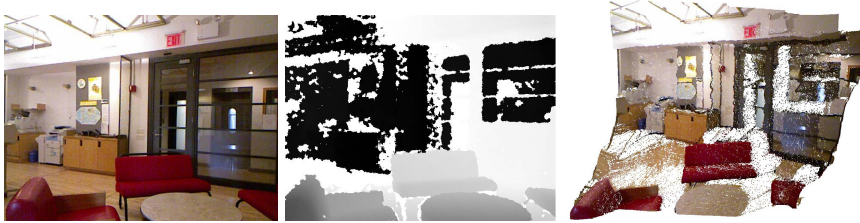
Fig. 5. Sample image from the dataset, associated raw depth map and the registered point cloud respectively
