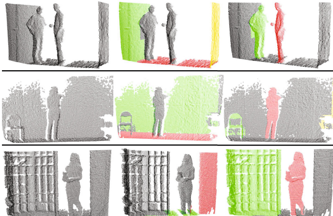
Fig. 4. Plane segmentation and obstacle detection results of three scenes. The first row is a sample of the corridor. The second is the classroom and the third is the office room. In each row, the first column is the original point cloud generated from depth images. The second column is the result of plane segmentation. Different planes are painted with different colors. The third column is the result of obstacle detection. Different obstacles are painted with different colors.
