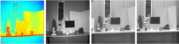
Fig. 2. Input data: TOFD, TOFI (200x200), L and R (1312x1082, cropped for vis.)
