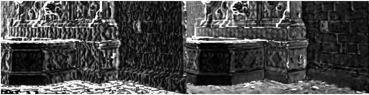
Fig. 6. Difference to ground truth. Left: No Normal Tuning Right: Tuning with random normals. Artifacts disappear nearly completely after the second propagation step.
