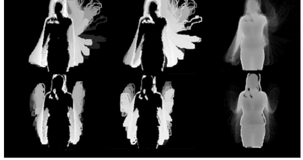
Figure 4. Illustration of the MHI , INV and GEI in two tokens (top row and bottom row). The projection images show that MHI emphasizes recent motion, i.e. ending frames whilst INV the beginning frames. GEI encodes the average gait information and is supplementary in repetitive actions where both MHI and INV are poor at representing.
