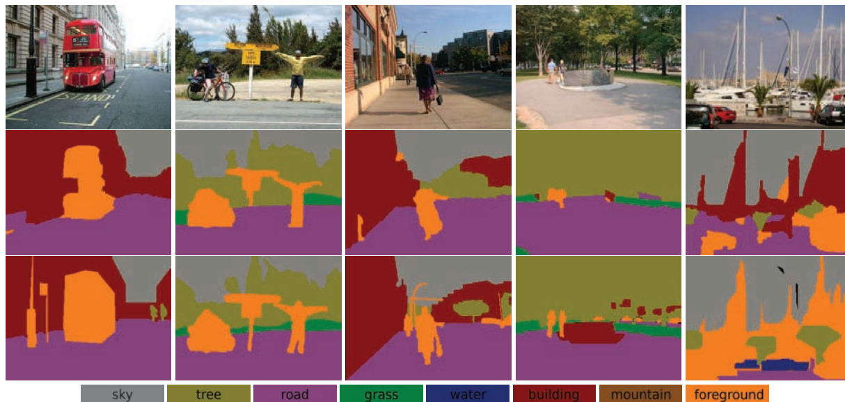
Figure 10. Examples of 8-class labeling results on the Stanford Background dataset. We do well in many challenging cases with large scale and appearance variations. The last example is interesting as discussed in [8]: we still confuse boat masts with building, but our segmentation is more accurate. (More examples can be found in the supplemental material.)
