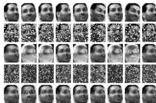
Figure 4. An example of DLRD_SR algorithm from UMIST database with 20% pixel corruptions. First row: original training images. Second row: corrupted training images. Third row: learned dictionary by DLRD_SR. Fourth row: separated noises from the second row by DLRD_SR. Fifth row: recovered images of the second row by DLRD_SR.
