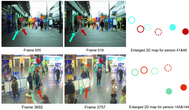
Figure 2. Examples of relative positions and linear estimations. In the 2D map, filled circles indicate positions of person at the earlier frames; dashed circles and solid circles indicate estimated positions by linear motion models and real positions at the later frames respectively.
