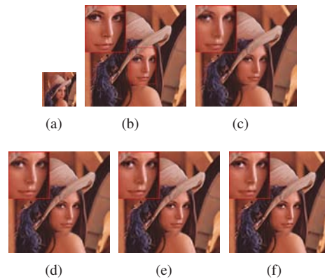
Figure 2. Reconstructed HR images (scaling factor 3) of Lena by different methods. Local magnification in red rectangle is shown in the upper-left corner in each example. (a) LR image; (b) original image; (c) SC; (d) SC-NLSS; (e) SC-Graph; (f) SC-NLSS-Graph.
