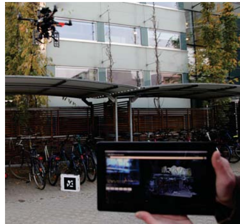
Figure 1. Our system is able to reconstruct a scene on-the-fly using a micro aerial vehicle. After automatic marker-based initialization, a live preview (left) and a live dense reconstruction (right) are streamed to a tablet for visualization. Best viewed in color.
