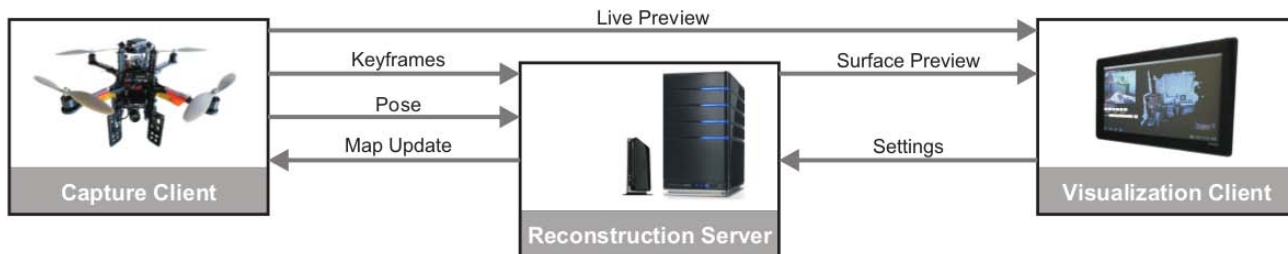
Figure 2. Overview of the distributed live dense reconstruction system, which exploits the individual capabilities and requirements of the system entities. The tracker is run on the quad-rotor, sparse and dense mapping on the server, and visualization on the tablet.
