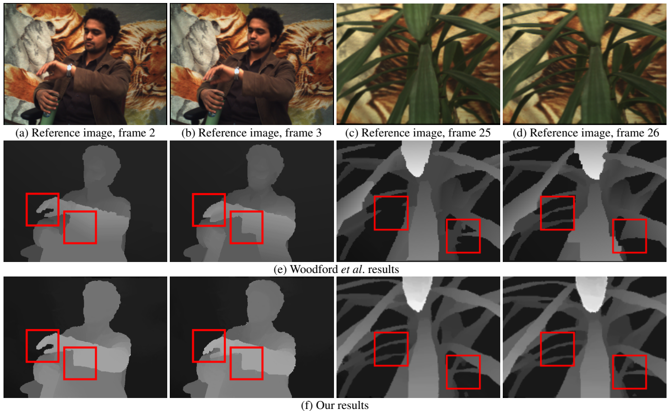
Figure 5. Depth results for two dynamic scenes using a five-camera. (a)-(b) Reference images from frames 2 and 3 of first scene. (c)-(d) Reference images from frames 25 and 26 of second scene. (e) Depth results obtained using Woodford et al. 's method [31]. (f) Depth results from our method. Note the improved temporal stability of our results, especially in the highlighted regions.
