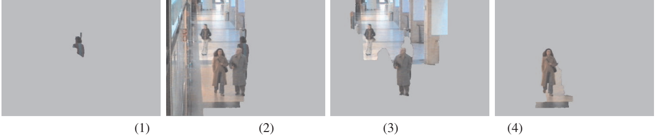
Figure 4. Four binary partition results got by the first 4 eigenvectors computed from motion profile (for one frame of the sequence WalkByShop1cor.mpg , CAVIAR database. ).
