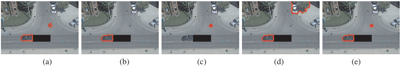
Figure 9. Segmentation results for the 16th frame of the car running sequence with occlusion. (a) The ground truth, (b) the result by the simple graph based segmentation using optical flow, (c) the result by the simple graph based segmentation using motion profile, (d) the result by the simple graph based segmentation using both motion cues, and (e) the result by the hypergraph cut.
