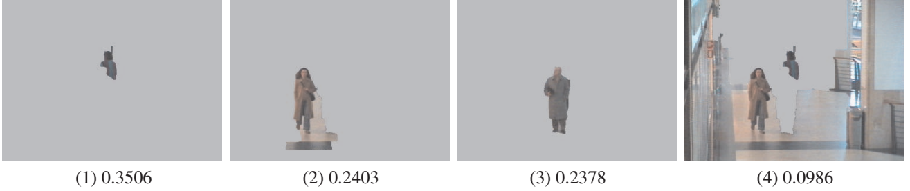
Figure 5. 4 binary partition results with largest hyperedge weights (for one frame of WalkByShop1cor.mpg ). Obviously that the hyperedge got from the 1st and 4th frames have a good description of objects we want to segment according to their importance. The computed hyperedge weights are shown below those binary images.
