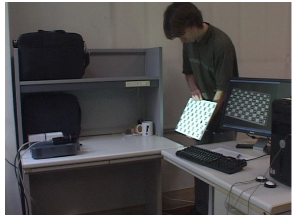
Figure 1. Snapshot of our demo video showing the test user calibrating a casually installed projector-camera system.
