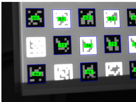
Figure 7. Lower left area of the detected markers from Figure 5. We can observe severe defocusing of projector markers.
