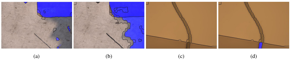
Figure 2: Role of segmentation. a) Failure due to inadequate Mean-shift segmentation, the shadow on the concrete is missed. b) Results with our segmentation for (a). c) Problematic case for our initial segmentation. d) Detection results of our method for image (c).
