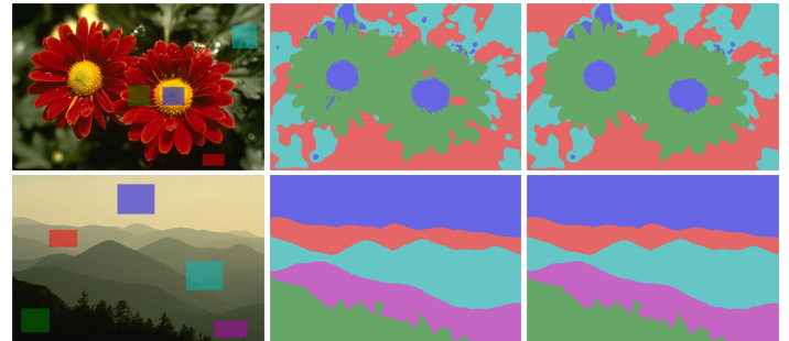
Figure 1: Comparison of our adaptive subdivision scheme to the large-scale quadratic program on standard image data. First column: input images, second column: labeling of the large-scale quadratic program, third column: labeling of our adaptive subdivision scheme for c = 5
