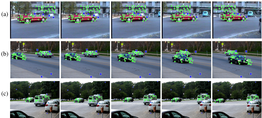
Figure 2: Three video sequences in Hopkins155. The marks \square and \times indicate feature point locations regarded as correctly tracked and incorrectly tracked, respectively, by our procedure.
