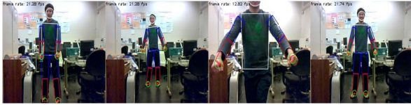
Figure 12: When the scale is so large that projected feet positions are out of camera range, only upper body tracking is used.
