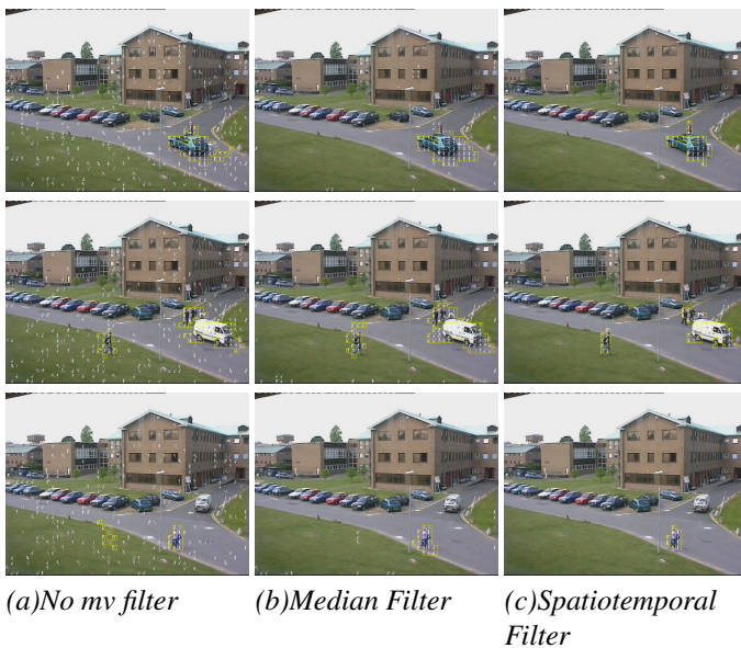
Figure 4. Object blobs and resulting motion vectors in sequence PETS2001 Camera1, using different motion-vector filters. Frames displayed: 570, 930, 2110
