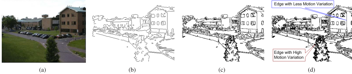
Figure 1. (a) A sample background reference image. (b) Edges from a single background reference image. (c) Edges from 25 superimposed background reference edge images. (d) Edges made from the accumulation of 50 superimposed background reference edge image.
