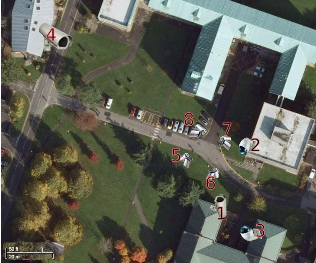
Figure 13. Plan view showing the location and direction of the 8 cameras on the Whiteknights Campus.
