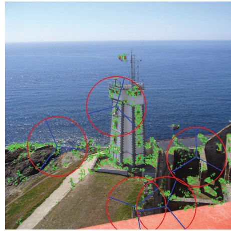
Figure 2: An example of spatial context of 5 random selected features. The green line means the dominate orientation of local feature and the red two pixel width circle represents the range of meaningful feature surrounding of the center feature. What’s more, the circle is parted into three parts by the blue two pixel width radius.
