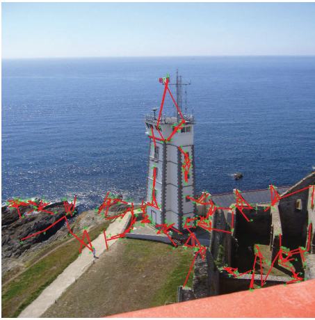
Figure 1: An example of some random selected feature tuples. The green arrow line means the dominate orientation of local feature and the red two pixel width line represents the pair of local features consisting of one feature tuple.
