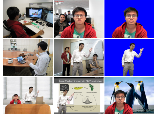
Figure 3: ITEM's real-time video object cutout technology using a normal webcam (top row) or a depth (plus RGB) camera (middle row). From left to right: system setup, input video frame, and cutout result. Bottom row shows some video composition effects.
