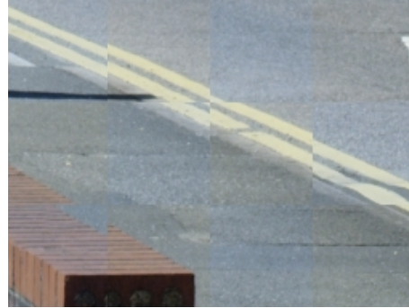
Fig. 8. Another close-up view, with alternating squares taken from the left and right views, further shows the colour differences that must be corrected in another portion of the scene.
