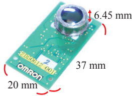
Fig. 4. Far-infrared sensor array used in the experiment. 16 \times 16 far infrared sensors are integrated in one chip.
