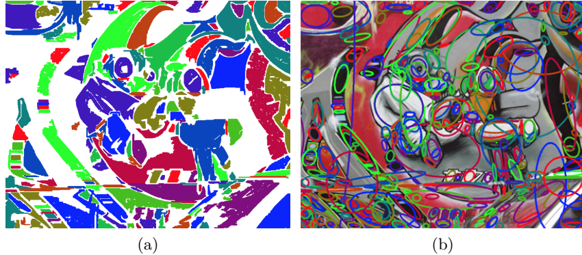
Fig. 1: Example of MSER detection. (a) Affine invariant regions detected by MSER. Each region is visualized as different color. (b) Each region is fit to elliptical shape.
