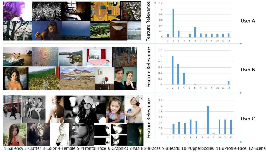
Fig. 7: Features weighted for three users and a sample of images they tagged as favorite. Users’ preferences can be represented using high-level visual features
