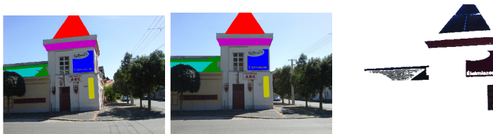
Fig. 7. 3D reconstruction result using MSER regions
