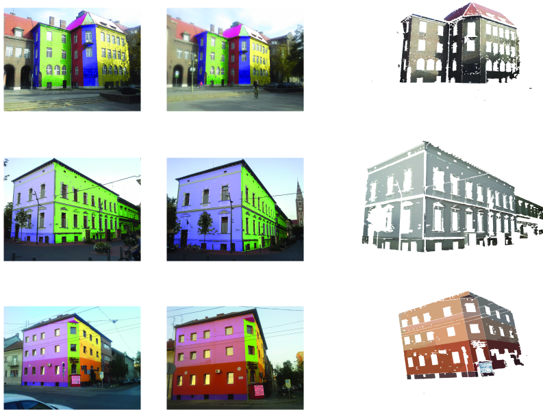
Fig. 8. 3D reconstruction results using regions extracted by color-based clustering
