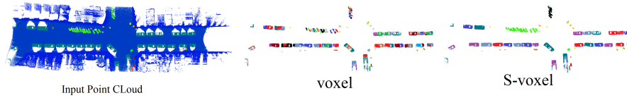
Fig. 4. Voxelisation of Point Cloud. from left to right: top view row point cloud, voxelisation result of objects point cloud after removing ground and building, s-voxelisation approach of point cloud
