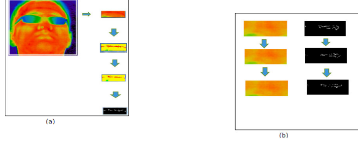
Fig. 13. (a) Segmentation of supraorbital area, white top hat segmentation, bilateral filter and binary image. Fig. 14. Detected blood vessel during stress area, white top hat segmentation, bilateral filter and binary image.
