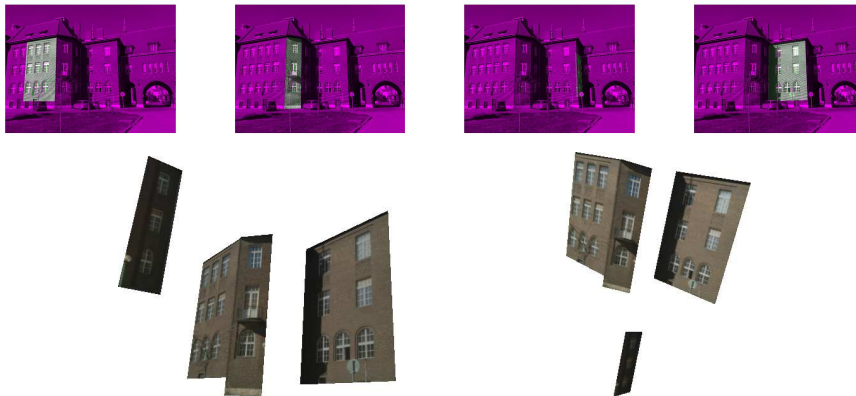
Fig. 3. Top: Initial patches of sequence No. 232. transformed by estimated homographies. The third one is an outlier due to failed patch registration. Bottom: Two views of the reconstructed 3D scene. The placement of the third planar patch is wrong but this can be detected by validating the homographies.
