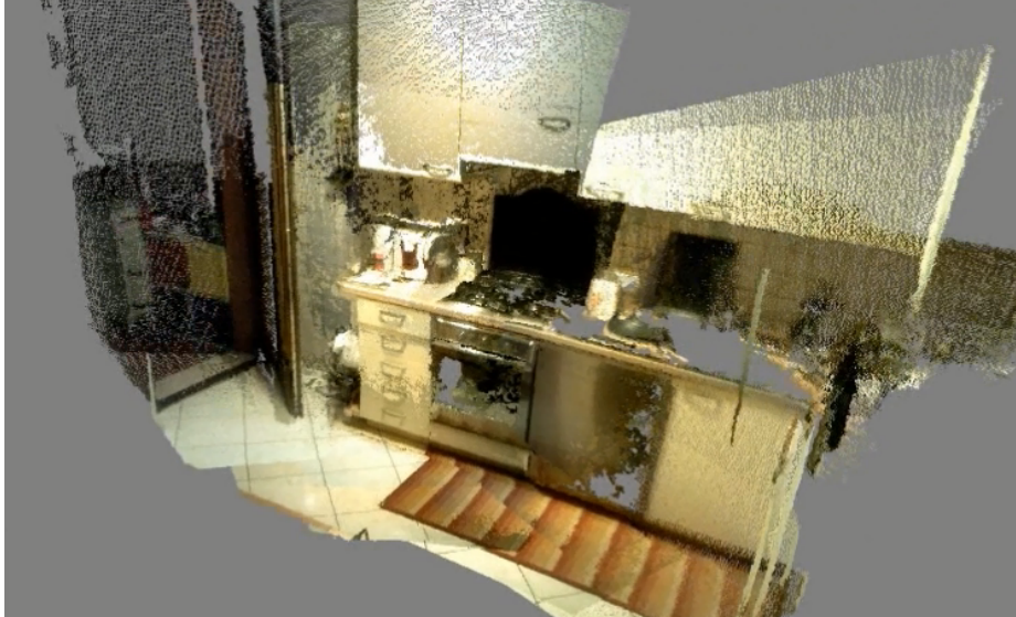
Fig. 4. 3D reconstruction of a kitchen using the Asus Xtion Pro Live camera.
