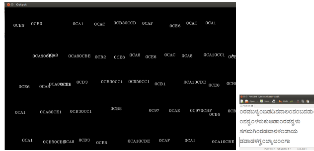
Fig. 8: An image with Unicodes at the locations of their respective characters (left) and the corresponding text image (right).
