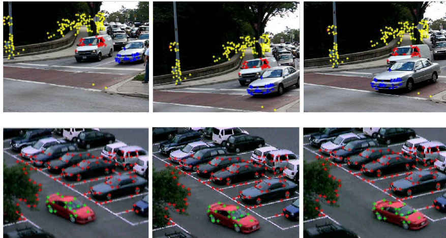
Fig. 1: Examples of our segmentation result on the real sequences cars9 and kananichi1 from the Hopkins155 dataset. (The first row: from left to right are the results for frame 1, 40 and 50; the second row: from left to right are the results for frame 1, 10 and 20.
