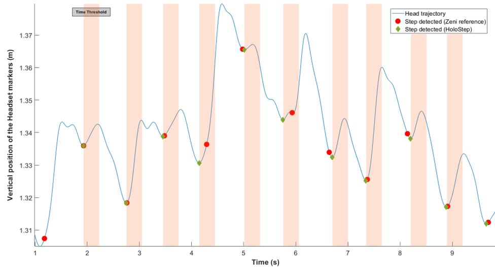
**Figure 3.** Representation of the locking time threshold. In blue, vertical head position  $y_F$  of the user wearing the AR HMD over the walkway. The green diamonds were the IC detected with HoloStep. The red circle were IC detected with Zeni algorithm reported to  $y_F$ . The orange bands were the locking time threshold (minimum peaks ignored by HoloStep).
