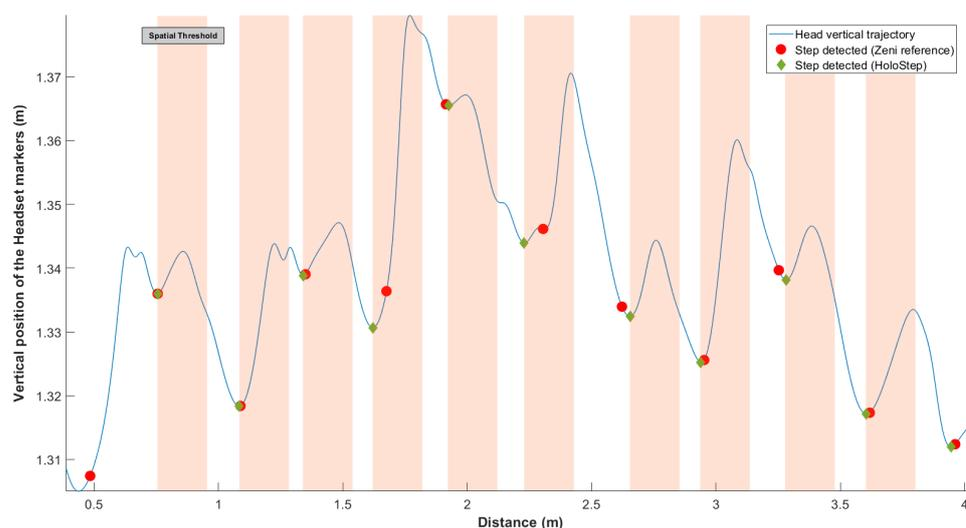
**Figure 2.** Representation of the locking distance threshold. In blue, vertical head position  $y_F$  of the user wearing the AR HMD over the walkway. The green diamonds were IC detected with HoloStep. The red circle were IC detected with Zeni algorithm reported to  $y_F$ . The orange bands were the locking distance threshold (minimum peaks ignored by HoloStep).
