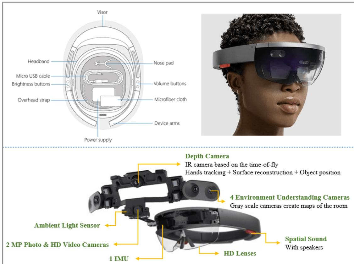
Figure 3.1 – Microsoft Hololens AR Headset. Top left: Basic features and accessories. Top right: Woman wearing the Microsoft Hololens (1<sup>st</sup> generation) used in our work. Bottom: Specifications of the Hololens
