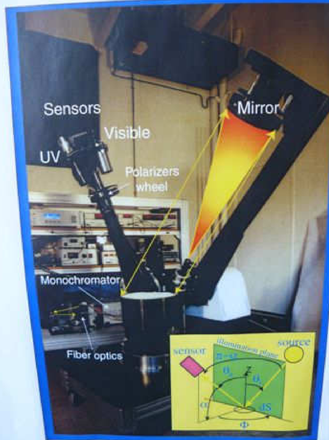
Fig. 1. Overview of the BRDF measurement setup
