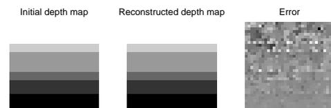
Figure 3 – Reconstruction results from 0.02% of the data ; different gray levels present different depths.
