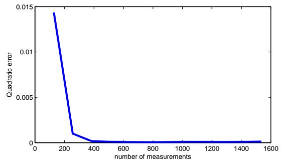
Figure 2 – Dependence of the error from the number of the measurements ; we see that roughly 400 measurements suffice to reconstruct a depth map of dimension  $128 \times 128$ .
