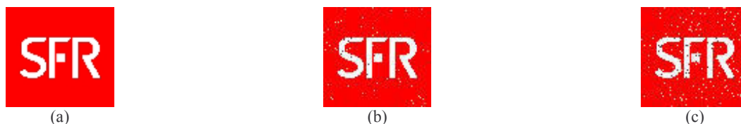
Figure 9 - Robustness for video watermarking: the SFR logo recovered after the file format changing (a), Laplace filtering (b) and the StirMark attack (c). Note that the logo (a) is practically identical to the original logo
