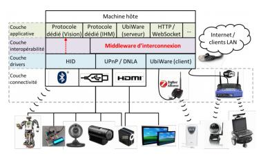
Figure 1: Preliminary architecture for the CIMA platform.
