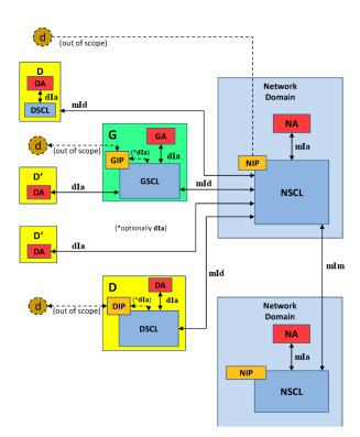
Figure 2: ETSI M2M reference Functional architecture (source: ETSI).
