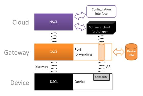
Figure 3: A schematic overview of the CIMA platform elements. (DIGIN)SCL are the different layers of the the OM2M framework.
